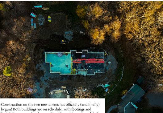
begun! Both buildings are on schedule, with footings and foundations poured and some plumbing and basement slabs in place for both. Crews have started framing the first floor and are moving toward closing up the greenhouse site for winter, and the Hepper House site is a few weeks behind that. Both dorms are on schedule to open in the fall of 2023, with the greenhouse site dorm being the first completed.
